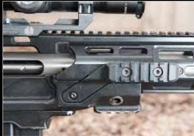
Side rails will accommodate lights and combat lasers, while the top rail will accommodate just about any type of scope.
